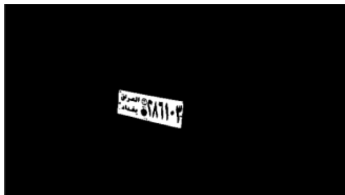
Fig. 7. Every point in the LP segment would be set to 1 in both TempA and TempB arrays
