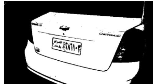
Fig. 3. LP candidate regions resulted from the proposed color closeness test operation
